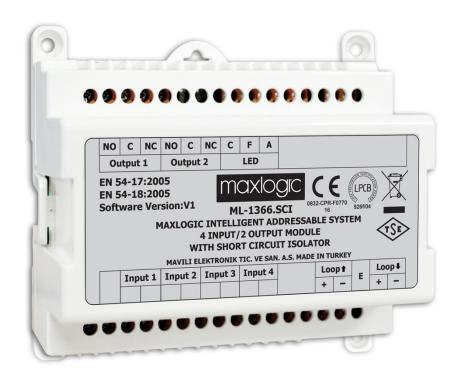
1 pc contact (volt free) monitor input. The device is loop powered. It can be programmed to operate in cause-effect scenarios. Within fire automation scenario with the help of switch monitor inputs any other system can be monitored and with the help of relay control outputs any other system can be controlled. Switch monitor inputs are used to monitor the outputs of dry (volt-free) contacts of relay output.
