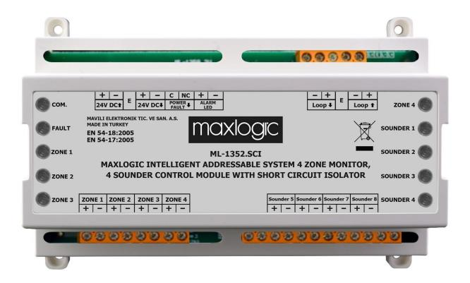
ML-1338, ML-1338.SCI (Short Circuit Isolated) I/O module with 8 Sounder Outputs, ML-1348, ML-1348.SCI (Short Circuit Isolated) I/O module with 8 Zone Monitoring Inputs, ML-1352, ML-1352.SCI (Short Circuit Isolated) I/O module with 4 Zone Monitoring Inputs and 4 Sounder Outputs. The modules require an external power supply of 18-30V DC. Relay outputs indicating fault conditions of the external power supply can be monitored. They can be programmed to operate in cause-and-effect scenarios.
