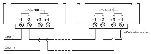
\* Resistor value is mentioned on panel. (MG / ML - 6K8)
